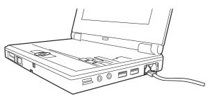
Sample connecting the telephone cable to the modem port
